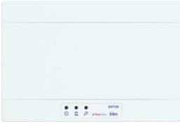
It is recognized on the loop as an Inim addressable device and occupies, in addition to its own, an address for each wireless device associated with it. The translator can manage directly up to a maximum of 32 wireless devices or, by adding XWT100 expansion modules, up to a maximum of 128 devices. It is powered via the Loop or via a local power source by connecting a 24 V power supply.
