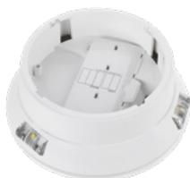
Occupies its own address in order to be managed independently by the detector it is associated with. It manages 32 different tones selectable via DIP switch and can be activated with two different tones (pre-alarm and alarm activation). The sounder base is compatible with the EWT100 addressable translators or the XWT100 expansions modules. The signaller can be used as a standalone ceiling-mount signaller (without detector) using the optional white or red cap.
