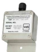
The ProReact EN Analogue End-of-Line Unit is a mandatory component in all ProReact EN Analogue LHD systems, as it plays a critical role in the proper functioning of the technology. It allows the control unit to detect any short circuits or breaks in the detector cable.
