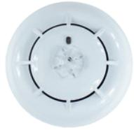
The detector can be set in the following modes: A1R (fixed threshold at 58°C with thermovelocimetric detection), B (fixed threshold at 72°C), A2S (fixed threshold at 58°C), BR (fixed threshold at 72°C with thermovelocimetric detection). As a result of its high flexibility, this detector is suitable for installation in dusty or smoky environments where the risk of false alarms is high.
