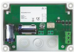
The WM202SR output module is equipped with a relay output (Dry contact) and a supervised output capable of supplying a voltage of 12 or 24 V DC starting from the internal battery. The module is completely managed by the control panel (if combined with addressed control panels).
