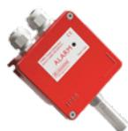
Absorption temperature sensor (for conventional control panels) TMP2-D series, aluminum enclosure with IP66 Protection Grade. 2 top cable entries, 2 M20 cable glands included. Automatic reset.
