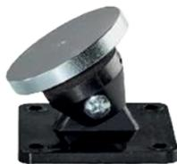
The counterplates of the S01 series use a steel disc mounted on a special shock damper capable of absorbing part of the impact caused by the opening of the door. The elasticity of the shock damper also allows for perfect alignment of the disc and magnet.
