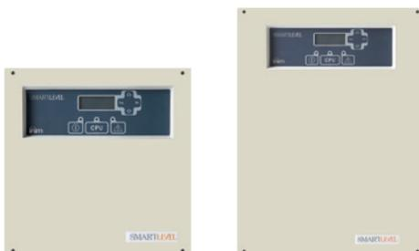
SPS24060S and SPS24160S power-supply stations (respectively 1.5A and 4A) with status LEDs, fault output, mains fault output, single power output. Can be used as a stand-alone device or connected directly to the loop of an addressable control panel (Inim protocol). Thanks to its loop interface, it is recognized by the control panel as being a power station and therefore becomes completely and automatically supervised thus reporting all signals to the control panel.
