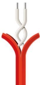
Thermocable's ProReact EN Digital Linear Heat Detection (LHD) cable uses fixed-temperature technology to easily and effectively detect temperature changes. This system represents a valid alternative for overheating protection in numerous contexts and places, such as tunnels, cable ducts, warehouses, escalators and other applications where potential fire risks can be hidden from view.
