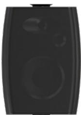
Wall mount two-way sound diffuser (5" speaker, 1.5" tweeter). Surface mount by means of the included metal coupling bracket, adjustable, flame-resistant ABS thermoplastic casing, metal grille for the protection of the visible section. Supports 70 V or 100 V lines, by means of a selector it can be set to provide a 7.5/15/30W power supply.
