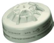
The conventional equipment of the Apollo Orbis I.S. proposed herein reaches the ATEX safety level by means of the "Intrinsically safe" technique. Intrinsically safe equipment operates at such low power and with such small amounts of stored energy that it does not constitute an ignition source under any operating conditions:
