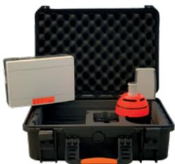
The case comprises: a test transmitter, a test detector, a Bluetooth adapter and a wireless transmitter for communication with Android APP. The kit allows the installer to carry out placement tests and evaluate the wireless signal before proceeding with the installation of the system. The wireless signal value transmitted by the test detector and test transmitter can be viewed on the App for android systems (smartphone-tablet) downloadable from the store.
