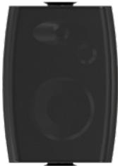
Wall mount two-way sound diffuser (4" speaker, 1" tweeter). Surface mount by means of the included metal coupling bracket, adjustable, flame-resistant ABS thermoplastic casing, metal grille for the protection of the visible section. Supports lines at 70 V or 100 V, by means of a selector it can be set to provide a 2.5/5/10 or 20W power supply.
