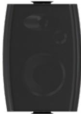
Wall mount two-way sound diffuser (6.5" speaker 1.5" tweeter). Surface mount by means of the included metal coupling bracket, adjustable, flame-resistant ABS thermoplastic casing, metal grille for the protection of the visible section. Supports 70 V or 100 V lines, by means of a selector it can be set to provide a 5/10/20/40W power supply.
