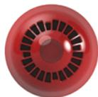
Optic section approved according new EN54-23 standard, complete with mounting base. Tone selectable from the 32 available by means of DIP switch, flash frequency 0.5Hz / 1Hz (selectable by means of DIP SWITCH), volume selectable from 2 levels.
