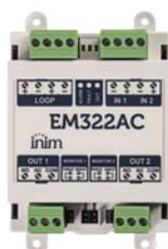
It connects to the loop and has two supervised inputs (capable of controlling the status of an external device) and two relays capable of driving mains voltage loads at 230V AC. For each of the two output relays it is possible to enable a supervisory function that allows you to check whether there is voltage across the contact when the relay is in stand-by status.
