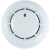
The ID100 optical smoke detector is based on the Tyndall effect (diffusion of light) and provides first-rate early warning in the event of fire. It offers wide-spectrum detection of smoke particles generated by the majority of fires. The newly designed optical chamber with sealed upper-part and 500 µm holes diameter mesh insect screen ensure high immunity to false alarms.
