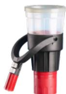
Can house inside SOLO A10 or SOLO A10S spray canisters (not included) and allows the delivery of the aerosol over the detector by simply exerting light pressure from the bottom upwards. Combined with the telescopic extension shown below, it allows the testing of detectors positioned as high up as 9m.
