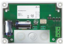
The WM110 input module is equipped with a supervised input and is compatible with EWT100 addressable translators or XWT100 expansions.
