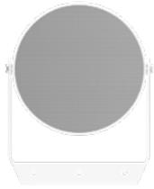
Projection-type sound diffuser. Assembly by means of the included metal coupling bracket, adjustable, flame-resistant ABS thermoplastic casing, metal grille for the protection of the visible section. Supports 70 V or 100 V lines, by means of a selector it can be set to provide a 5/10/20 W power supply.
