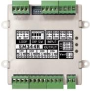
The module connects to the loop and provides different inputs and outputs depending on the model (see table). In the versions equipped with 4 inputs, 2 of these can be configured as conventional zones or 4-20mA inputs, powered by the Loop or by a local power source. The 4 outputs are, depending on the model, supervised for the management of audible/visual signallers or dry contacts.
