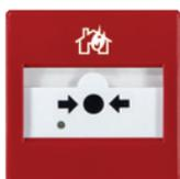
Resettable call point, can be connected to the loop and managed by analogue-addressable fire control panels. The device trigger element and red status LED are located in the front of the device casing. After activation the call point can be reset by means of the reset key included in the package.
