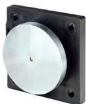
The counterplates of the S02, SH2, S00 series use a steel disc mounted on a special shock damper capable of absorbing part of the impact caused by the opening of the door. The elasticity of the shock damper also allows for perfect alignment of the disc and magnet.
