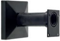
Extension S03130 for S2 electromagnetic door holders, used in cases where the electromagnet installed on the wall is too far from the door to be held. The extension allows an increase in the distance between the electromagnet and the wall of from 45 to 130 mm and, by adding the accessory rod, reach 230 mm. For medium distances, the rod can be shortened by cutting it to size, the S03130 extension is UNI EN 1155 certified for all S2 electromagnets with 50 or 100 Kg holding force.
