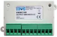
Argus series modules allow status monitoring of external devices (input modules) or control of external devices or actuators (output modules). The modules include a short-circuit isolator and are available in Mini (96 x 52mm) or Wall (86 x 86mm) version
