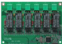
The SmartLoop/INOUT expansion board adds a further 6 terminals to the control panel. Each terminal can be set up to operate as either a supervised output NAC (1A max.); supervised input or input line (zone) for conventional detectors. The output trigger signals and the actions generated by the activation of the inputs are fully programmable.
