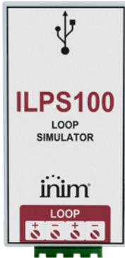
Connects to the Loop terminals of Inim control panels and simulates up to 240 devices, allows testing of loop functioning, verification of configuration and the cause/effect activation logics without having to physically connect the devices. Connects to a PC via the USB port (electrically decoupled so as not to interfere with the control panel and generate earth faults) and thanks to the "ILP Simulator" software it is possible to:
