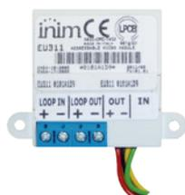
Thanks to its reduced-size it can be housed directly inside the enclosure of the device it controls (call point, sounder/flasher, beam detector, etc.), it connects to the loop and has a supervised input (to control the status of a device) and an output powered directly by the Loop (to drive a signalling or audible/visual signalling device).
