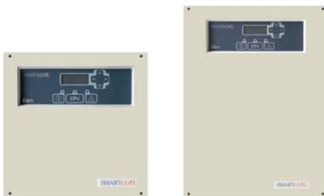
SPS24060G and SPS24160G (respectively 1.5A and 4A) with LCD command screen for viewing the events log or fault details (low battery, mains failure, dispersion to earth, etc.) and the current draw of each output; provides 3 individually protected outputs with 4A current limit.
